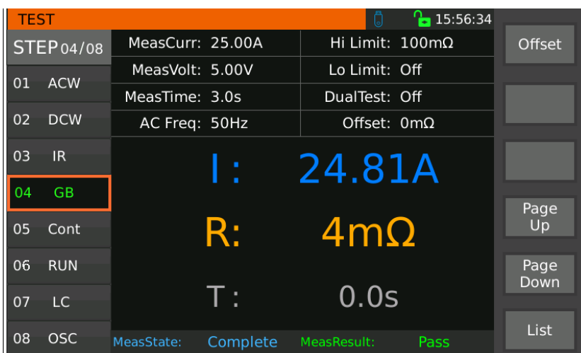
Figure 3-36.4 Grounding Resistance Measurement
