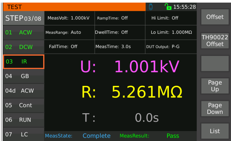
Figure 3-36.3 Insulation Resistance Measurement
