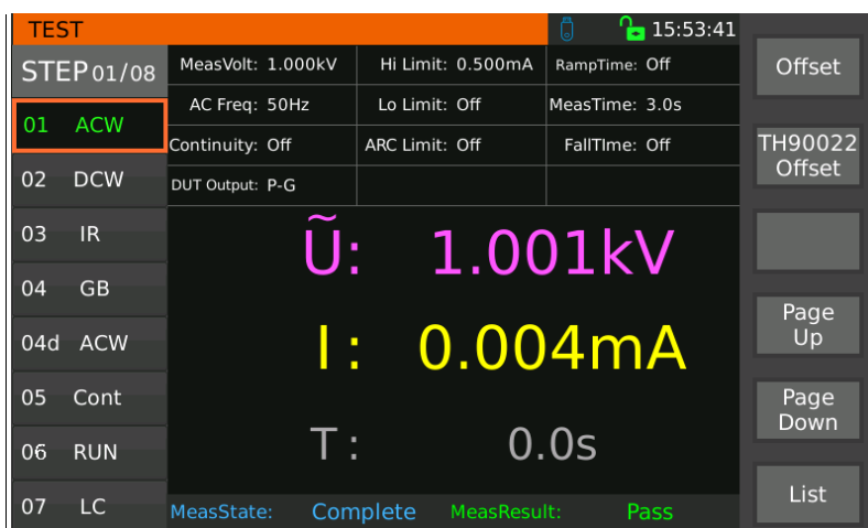
Figure 3-36.1 AC Withstand Voltage Measurement
