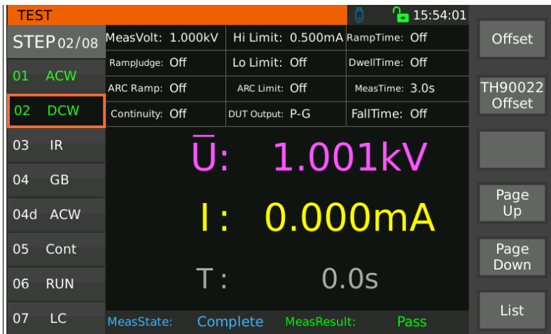
Figure 3-36.2 DC Withstand Voltage Measurement
