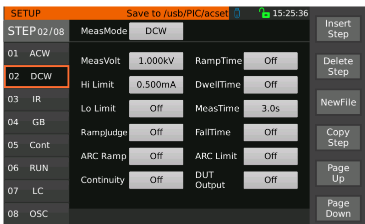
Figure 3-17 DC Withstand Voltage Setting
