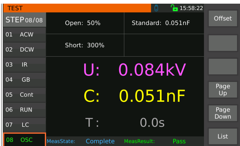
Figure 3-36.8 Open/Short Circuit Measurement
